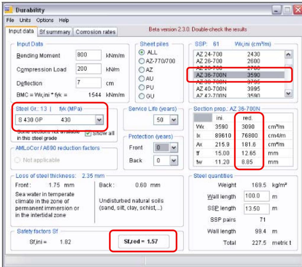
Total loss of steel thickness: 2.35 mm.
