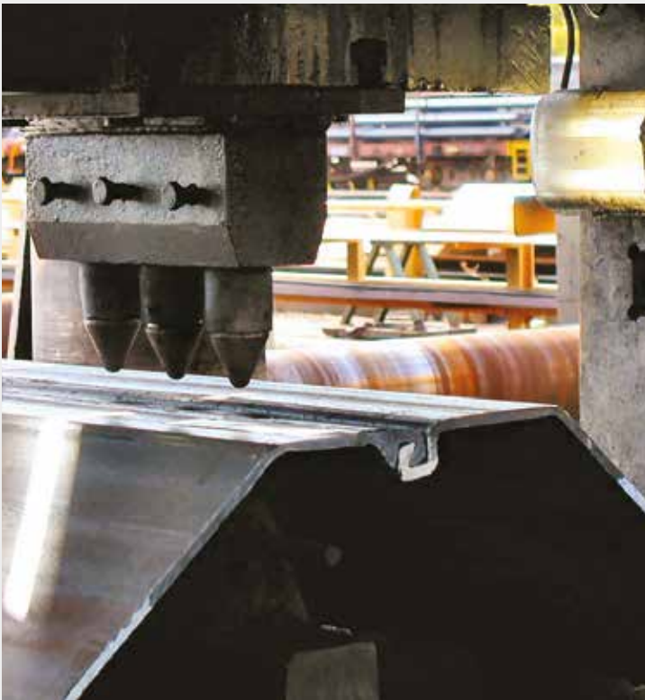
Fig. 8. Special crimping pattern for AZ infill sheet piles and crimping at the rolling mill.
