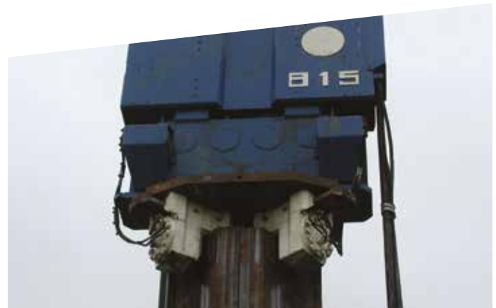
Fig. 13. Double clamps for a vibratory hammer.
