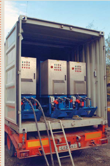
For long sheet pile structures, it may be very economical to use a truck-mounted container housing the pumps.
