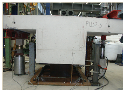
Picture 7. PU 32 during a loading test.
