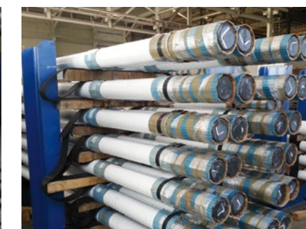
Storage of wrapped anchors
