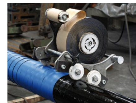
Factory wrapping of anchors
