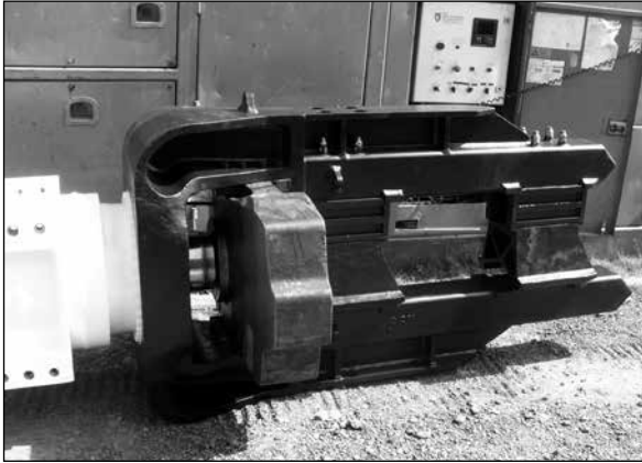
Fig. 11.9. Hydraulic hammer and anvil plate.
