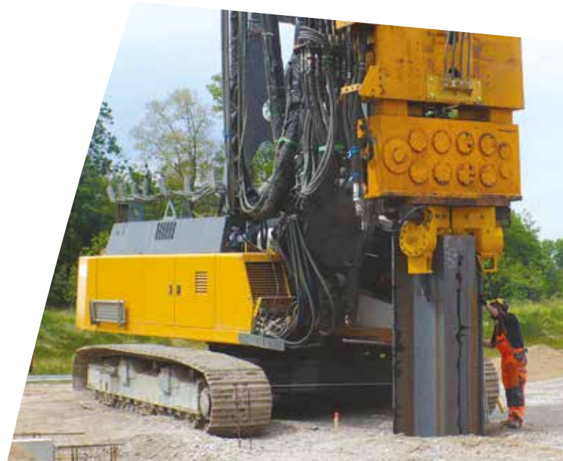
Leader-mounted vibratory hammer with double clamps.
