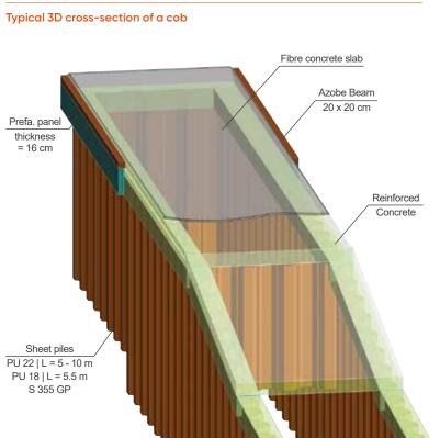
The long-term success of the project relies on regular site maintenance, including periodic recharging of the pebble beach. The groynes were built using PU 12, PU 18, and PU 22 steel sheet piles, with lengths ranging from 3.8 to 10.0 meters, in steel grade S 355 GP. The sheet piles were capped with a reinforced concrete beam topped by an exotic hardwood edge made of Azobé.
