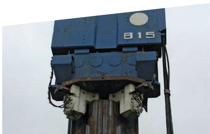
Fig. 20. Double clamps for a vibratory hammer.
