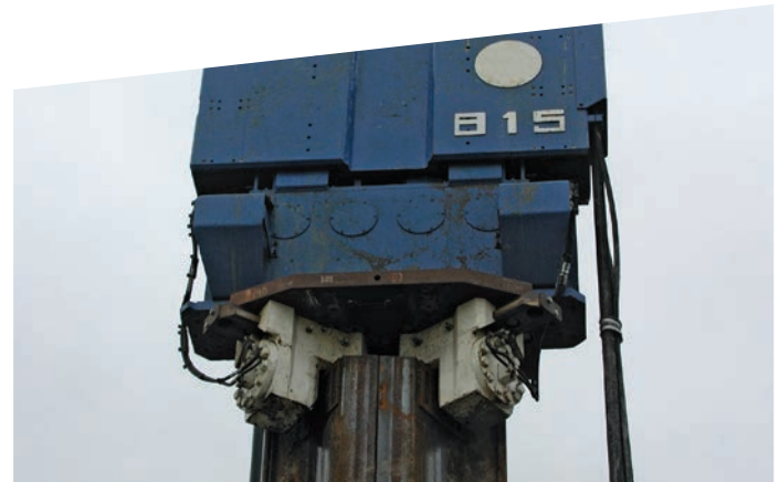
Fig. 20. Double clamps for a vibratory hammer.
