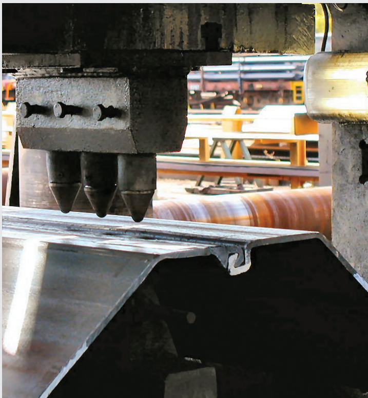
Fig. 15. Special crimping pattern for AZ infill sheet piles and crimping at the rolling mill.
