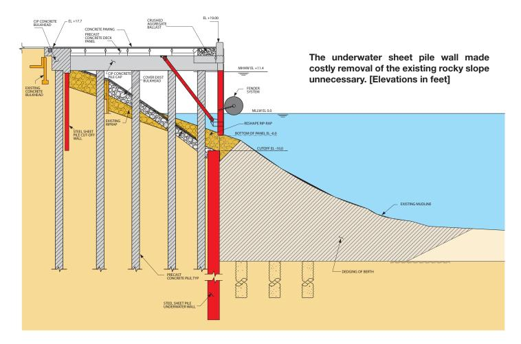
the underwater steel sheet pile wall at the end of the rocky slope. The contractor, M.A. Segale Inc., fabricated his own template for the installation of the HZ 975 D - 24 / AZ 19 combined-wall system. A total of 1,315 t of sheet piles in a high steel grade were delivered to the site.
