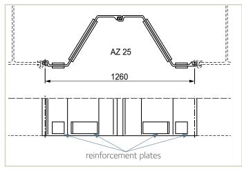
The toe of the double AZ pile was reinforced with 15-mm-thick steel plates.
