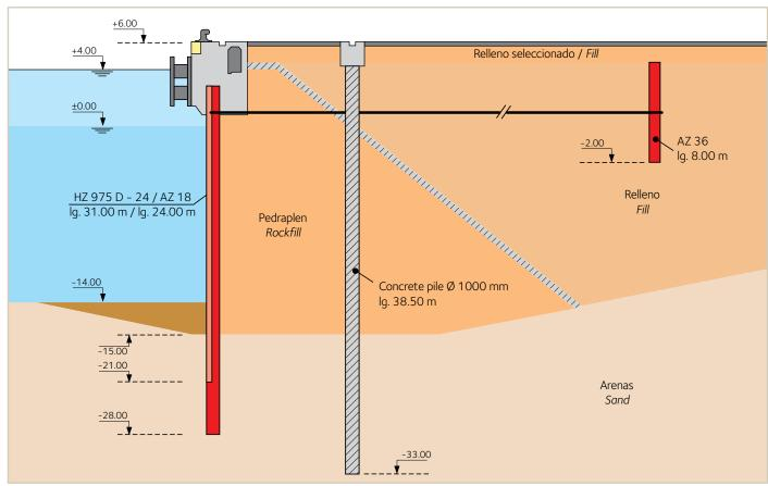
A combined steel sheet pile system was used to build the 20-m-high guay wall.
