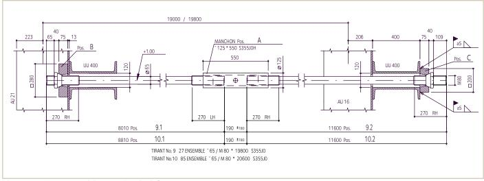
The 65-mm-diameter tie rods have a working load of 680 kN.
