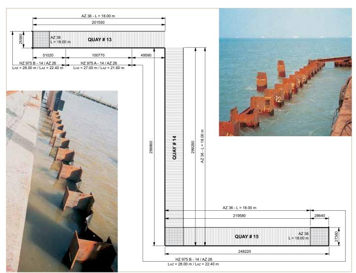
The Formosa Plastics Corporation required three new quays. Due to its advantageous installation speed, the choice fell in favour of the HZ/AZ combined-wall system.
