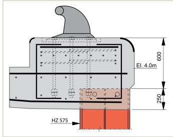
Steel sheet pile - capping beam connection detail with bollard.
