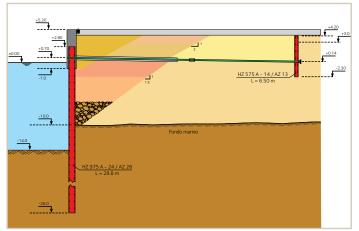
Typical cross-section of the HZ/AZ system adapted to the varying water depth.
