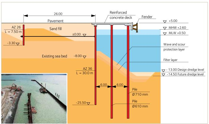
The originally planned HZ/AZ quay wall was replaced by a more economical AZ 36 wall.
