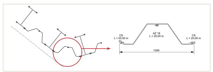
C9 connecters welded to an AZ 18 double pile formed the corner of the segmented quay wall.
