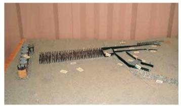
The breakwater consists of sheet pile cells assembled with straight-web sections, whereas bending-moment-resisting sheet piles were used to build the terminal walls.
