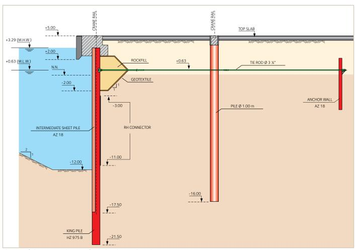
The state-of-the-art terminal consists of an anchored HZ/AZ sheet pile system.
