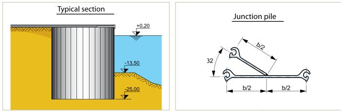
Cross-section of the AS 500 sheet pile cell.
