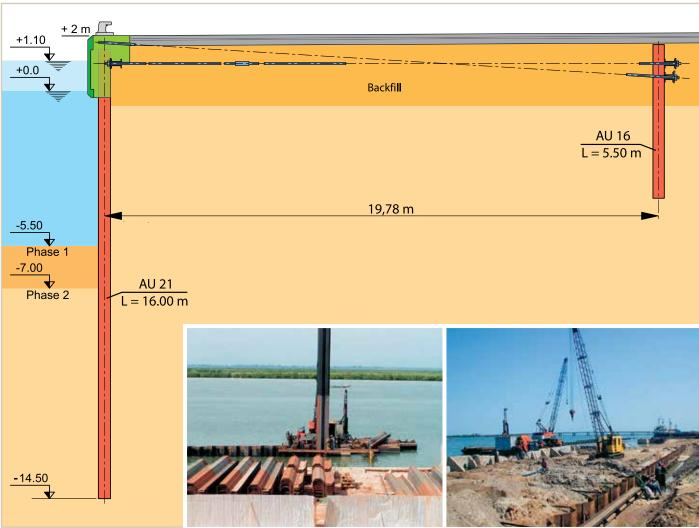
The new quay wall was built with AU 21 sheet piles driven 20 m in front of the dilapidated structure.
