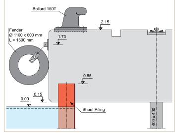
Concrete capping beam showing fender, bollard, crane rail and top of sheet pile.
