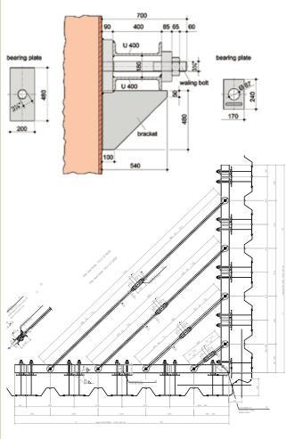
Tie-rod system – Details of the quay wall corner.
