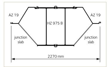
The double king piles and the intermediary piles were delivered to the site as joined elements.
