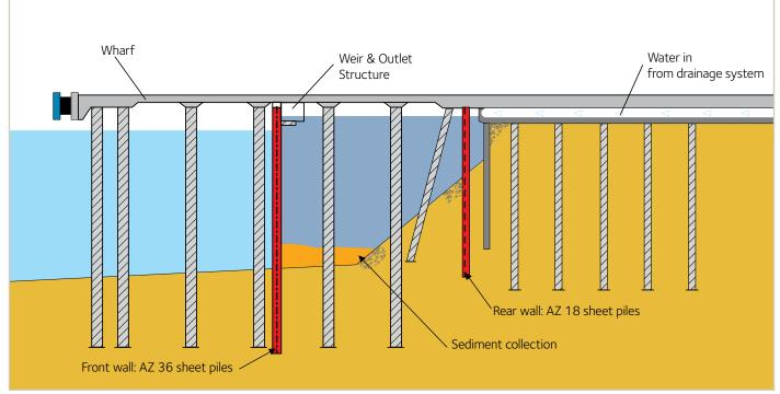
Cross-section of the expanded terminal with the stormwater detention basin set between two rows of AZ sheet piles.
