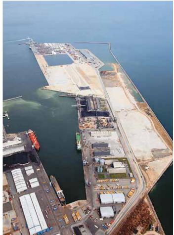
Some 3.5  $\text{Mm}^3$  of sand were placed behind the sheet pile wall to create the new CT East.
