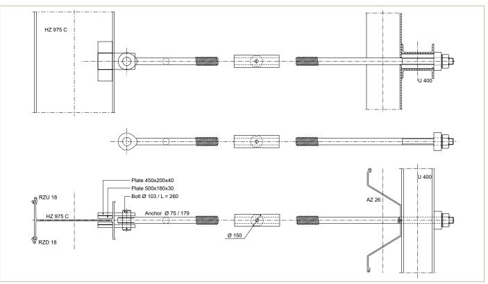
Two different sets of upset tie rods were used, depending on the HZ/AZ system chosen.
