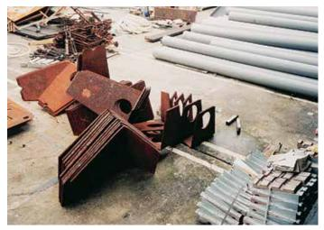
L-shaped plates were used to connect the sheet piles to the anchors.
