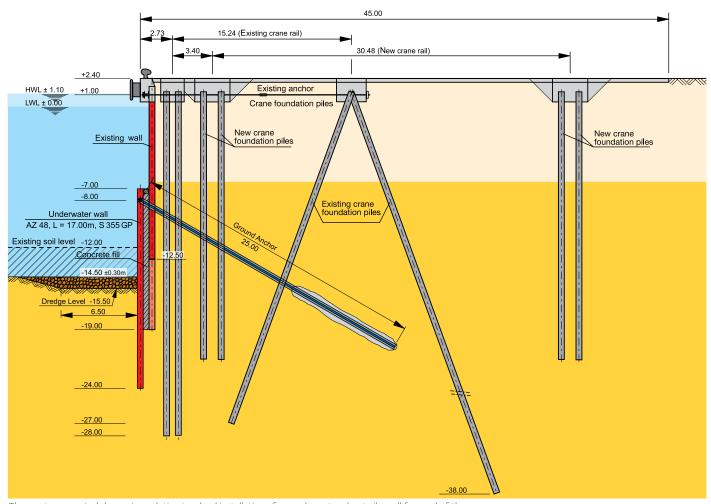
The most economical deepening solution involved installation of an underwater sheet pile wall forward of the quay.
