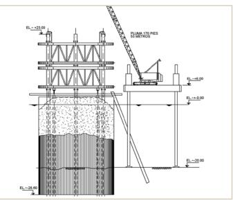
Removal of the template and filling of the cells.
