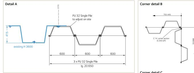
The existing sheet piles were connected to the new PU 32 sheet piles by a single pile that was adjusted on site.
