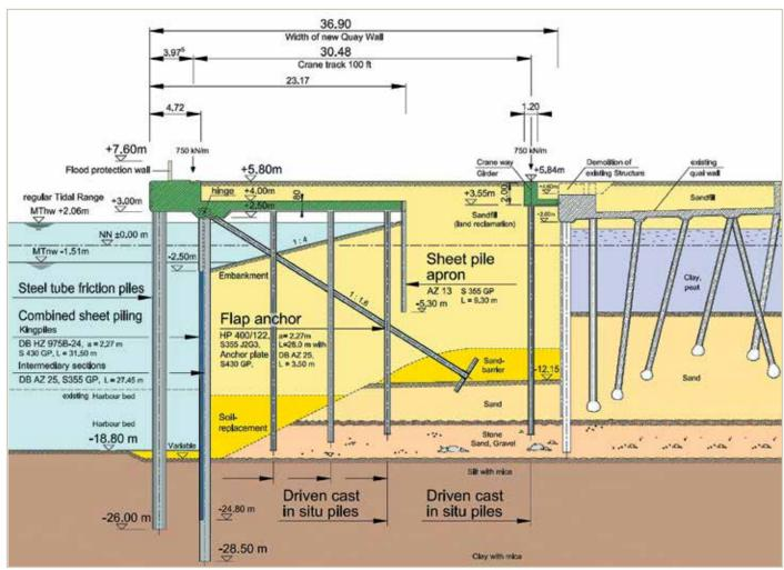
The quay wall consists of a high-strength HZ 975 B - 24 / AZ 25 sheet pile solution.
