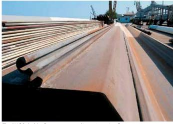
The AU 20 double piles were arranged into a jagged wall using Omega 18 connectors.
