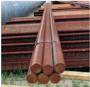
The tie rod consists of a 28 m steel bar, 56 or 63 mm in diameter.
