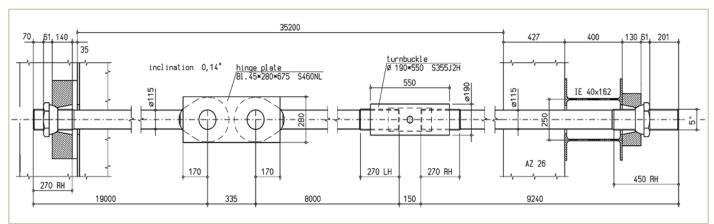
The steel tie rod is in three parts to facilitate transportation.
