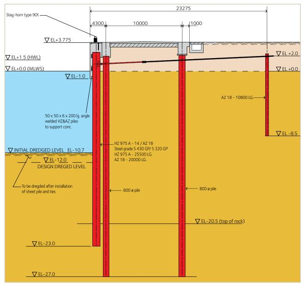
The HZ 975 A - 14 / AZ 18 main wall is installed 23 m in front of the AZ 18 anchor wall.
