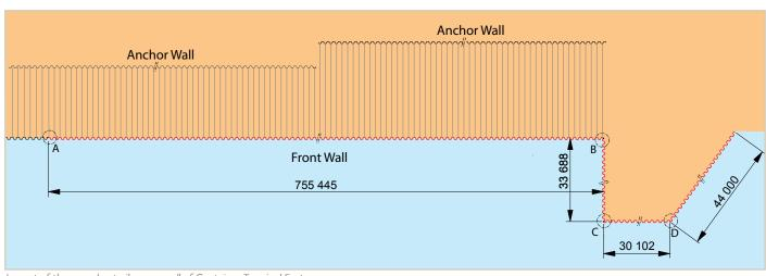
Layout of the new sheet pile quay wall of Container Terminal East.
