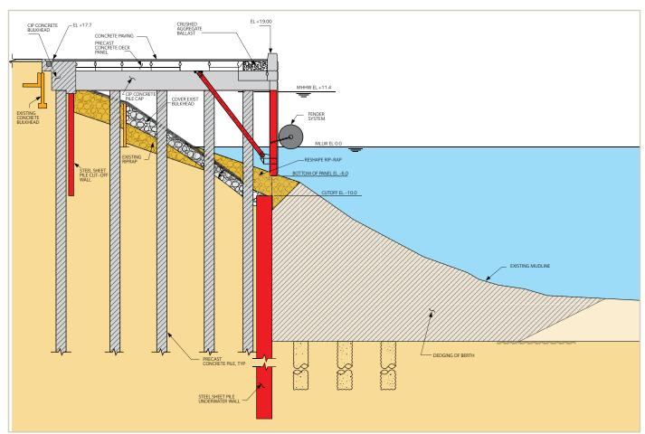
The underwater sheet pile wall made costly removal of the existing rocky slope unnecessary. [Elevations in feet].
