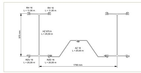
The combined wall was locally reinforced with RH sections.
