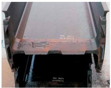
Driving shoes protect the pile toe from damage when hard soil layers are expected during driving.
