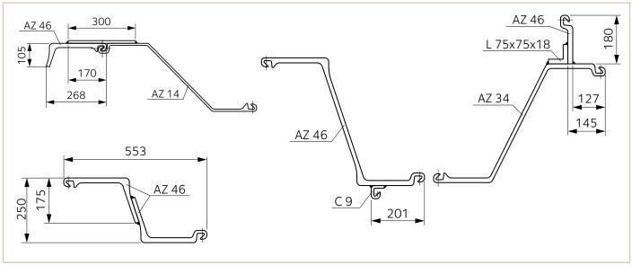
Several special piles were used to connect the different wall axes.
