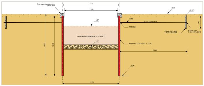
ArcelorMittal supplied AZ 17 sheet piles in six different lengths for the trench.
