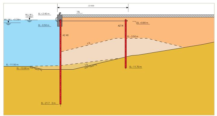
The AZ 46 sheet piles of Quays 1 & 2 were installed 52 m in front of existing berths.
