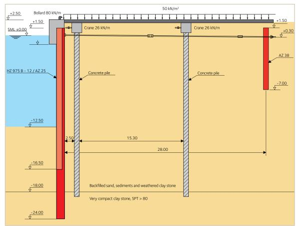
Cross-section: combined HZ/AZ main wall anchored with an AZ 38 wall.
