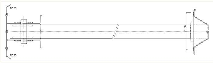
Pivoted tension piles welded to AZ 25 sheet piles acted as anchors.
