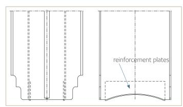
The web and flanges of the king piles were cut to facilitate penetration into the hard soil.
