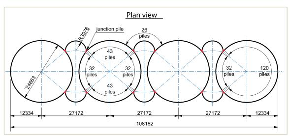
The wharf consists of four cells and six connecting arcs.
