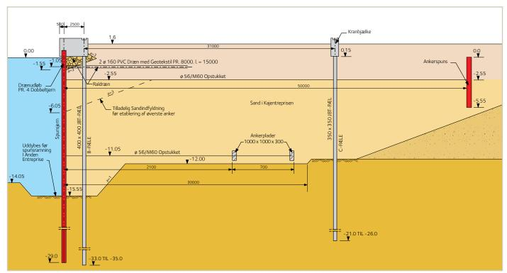
Two levels of tie rods were chosen due to poor soil conditions leading to the positive side-effect of reducing maximum bending moments. A combined wall system was thus unnecessary. The underwater installation of tie rods by divers was a complex task however.
