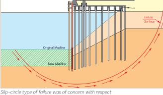
sup-circle type of failure was of concern with respec to the stability of the new wharf.
