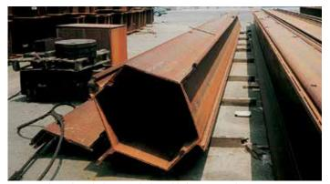
A CAZ 36 box pile with three interlocks welded on was used where the anchor walls intersect.
