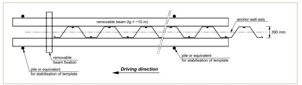
A second driving template facilitated installation of the AZ 18 anchor wall.
