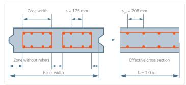
Figure 3.4. Rebars in diaphragm wall, ø32/206 (tension)+ø20/206 (compression).
