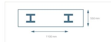
Figure 3.8. SoilMix wall with HEA 320 insert.
