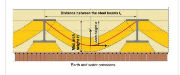
Figure 3.9. Working principle of a soil mix retaining wall; illustration of the arching effect.
