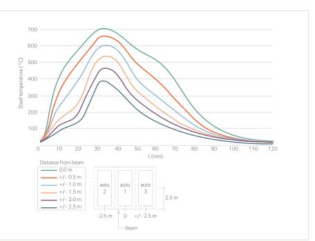
Figure 4.1. Fire load per car, scenario three car fire, Eurocode 3. A.F. Hamerlink.
