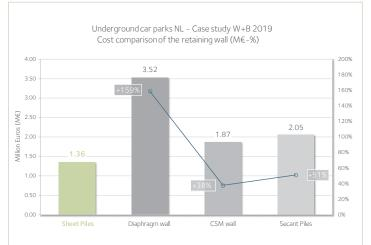
Figure 5.1. Cost estimate of the retaining wall per alternative.
