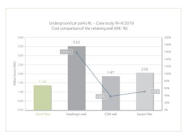
In this case study, the steel sheet pile solution is at least 38 % more cost-effective for the retaining wall of the Underground Car Park with 2 levels below grade.
