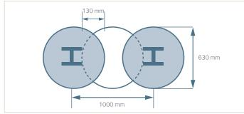
Figure 3.14. Secant pile wall with HEA 320 inserts.
