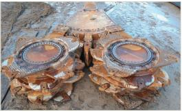
Figure 3.10. Cutting tool and injection point SoilMix.
