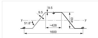
Figure 3.1. Sheet pile profile AZ 20-800.
