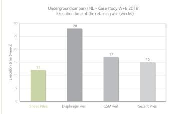
Figure 5.2. Execution time of the retaining wall per alternative.
