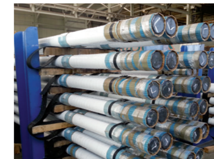
Storage of wrapped anchors
