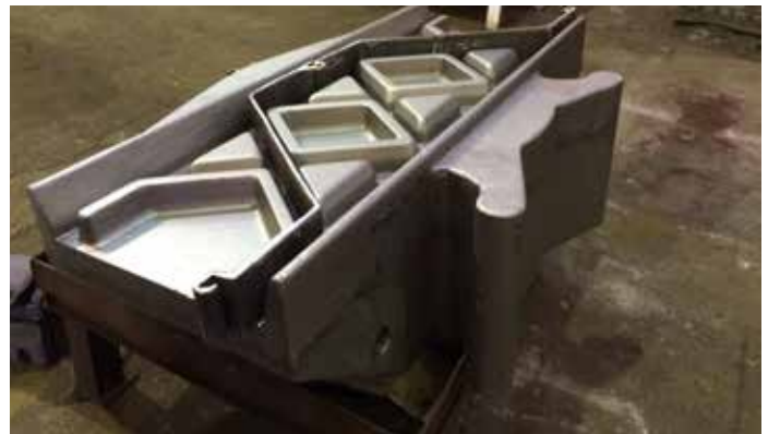
Driving cap for impact hammer.
